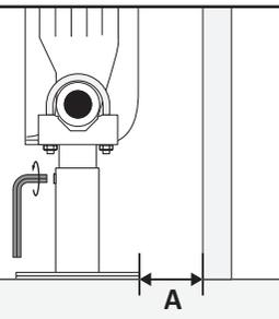
A = Distance mounting feet / wall : 30mm for standard and low model Neomitis electric radiators, 40mm for slim Neomitis electric radiators.
